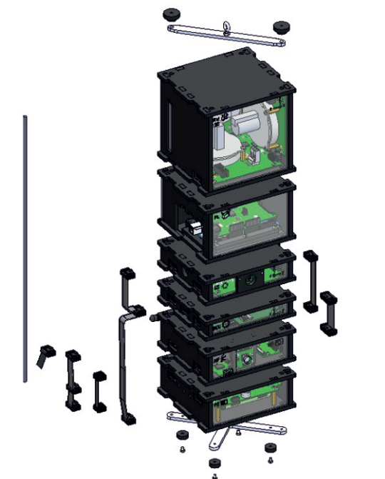
Fig. 107: Assembling an OrbiCraft 3D in a three-axis configuration
