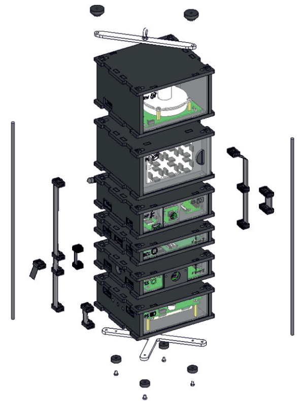
Fig. 101: Assembling an OrbiCraft 3D in a uniaxial configuration
