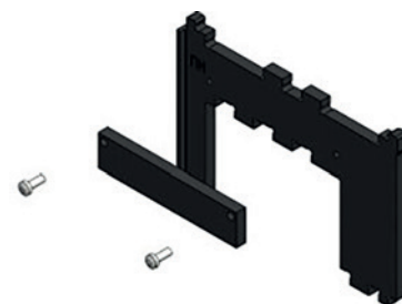
Fig. 40: Securing a detent to the side wall
