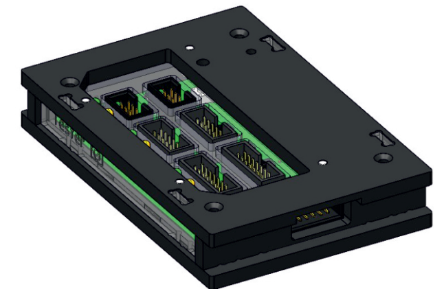
Fig. 88: Installing the top cover
