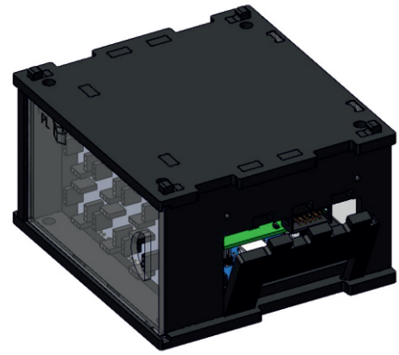
Fig. 46: Mounting the side cover
