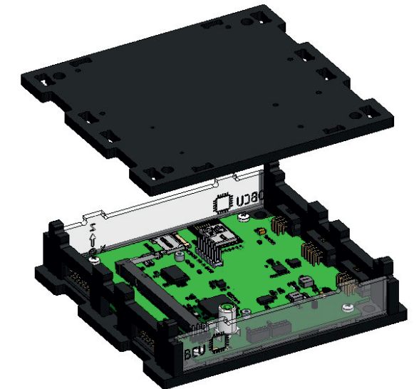
Fig. 21: Installing the top cover
